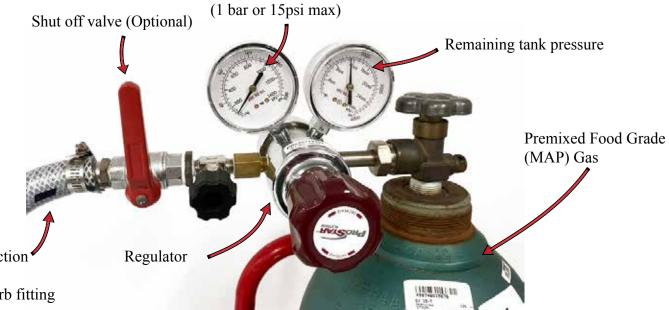
Gas Hose Connection to machine. Use same size barb fitting as shown above.
